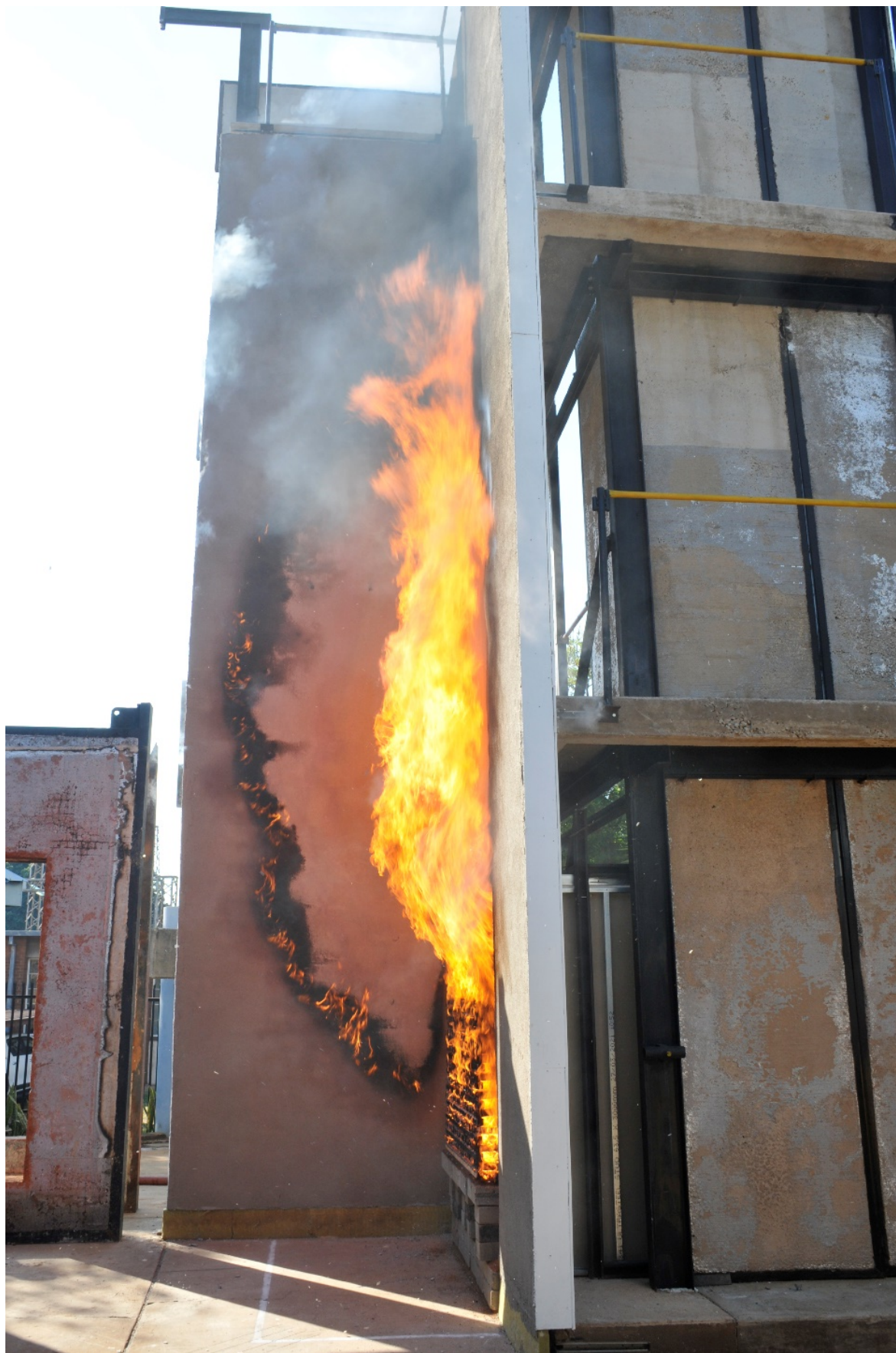
Figure 3.11: Surface flame spread beyond confines dimension (1.5 m)
