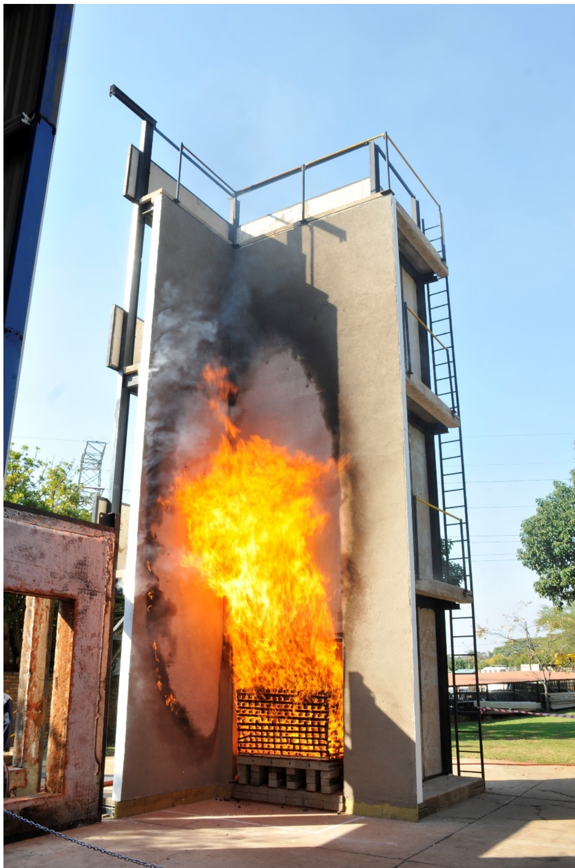
Figure 3.12: Smoke release from Wing Wall's edges
