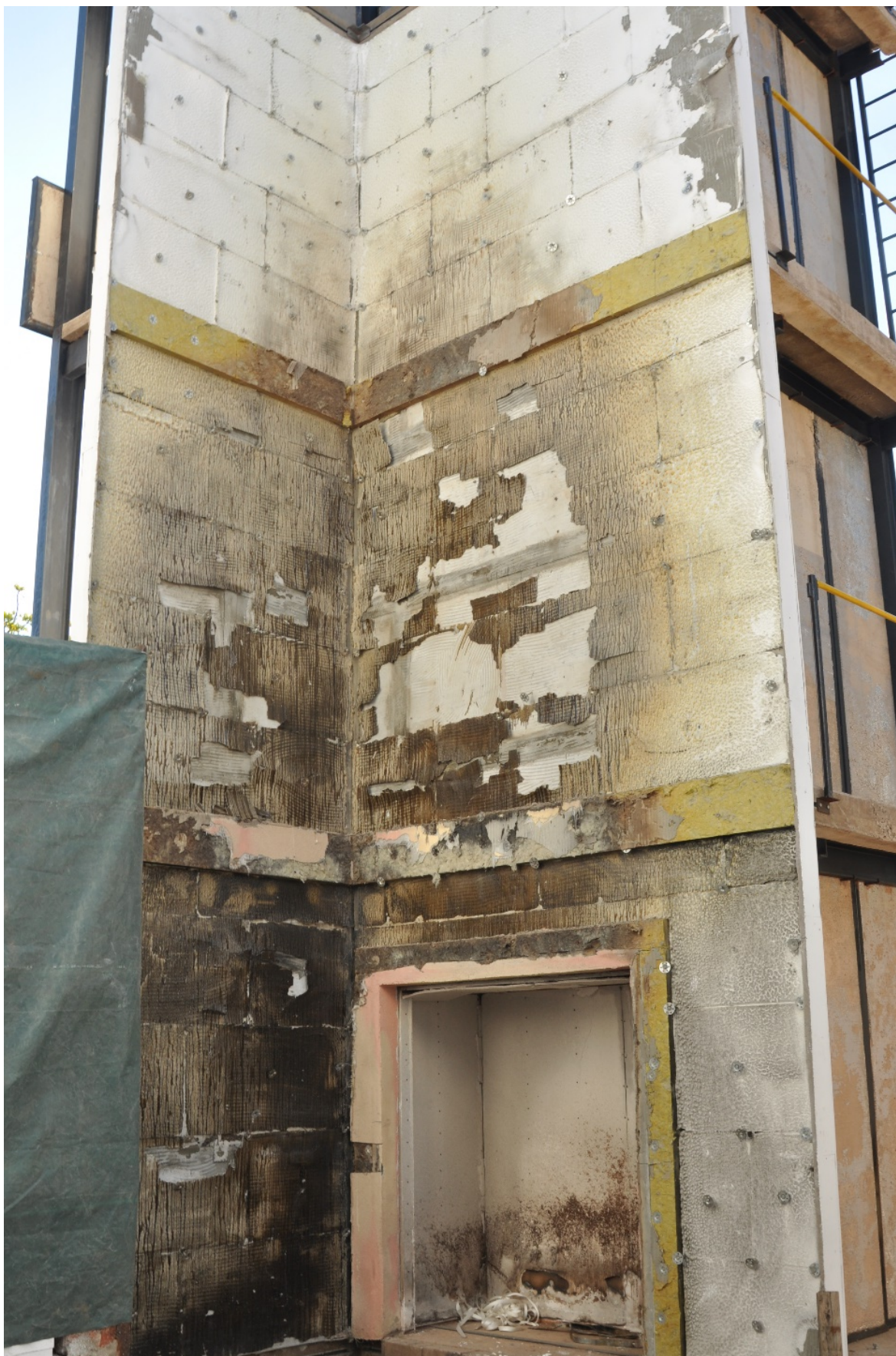
Figure 4.1: Specimen after removal of external coat
