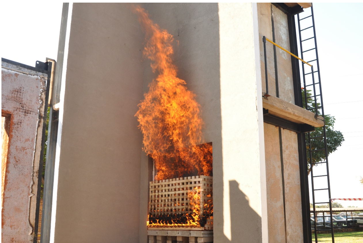
Figure 3.6: Flames extending up to Level 1
