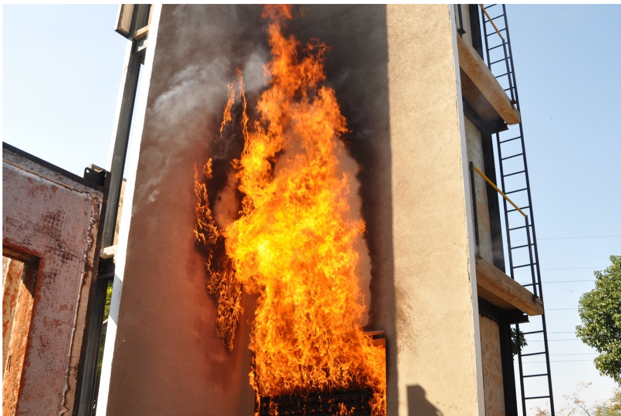
Figure 3.9: Flaming and discolouration on Wing Wall
