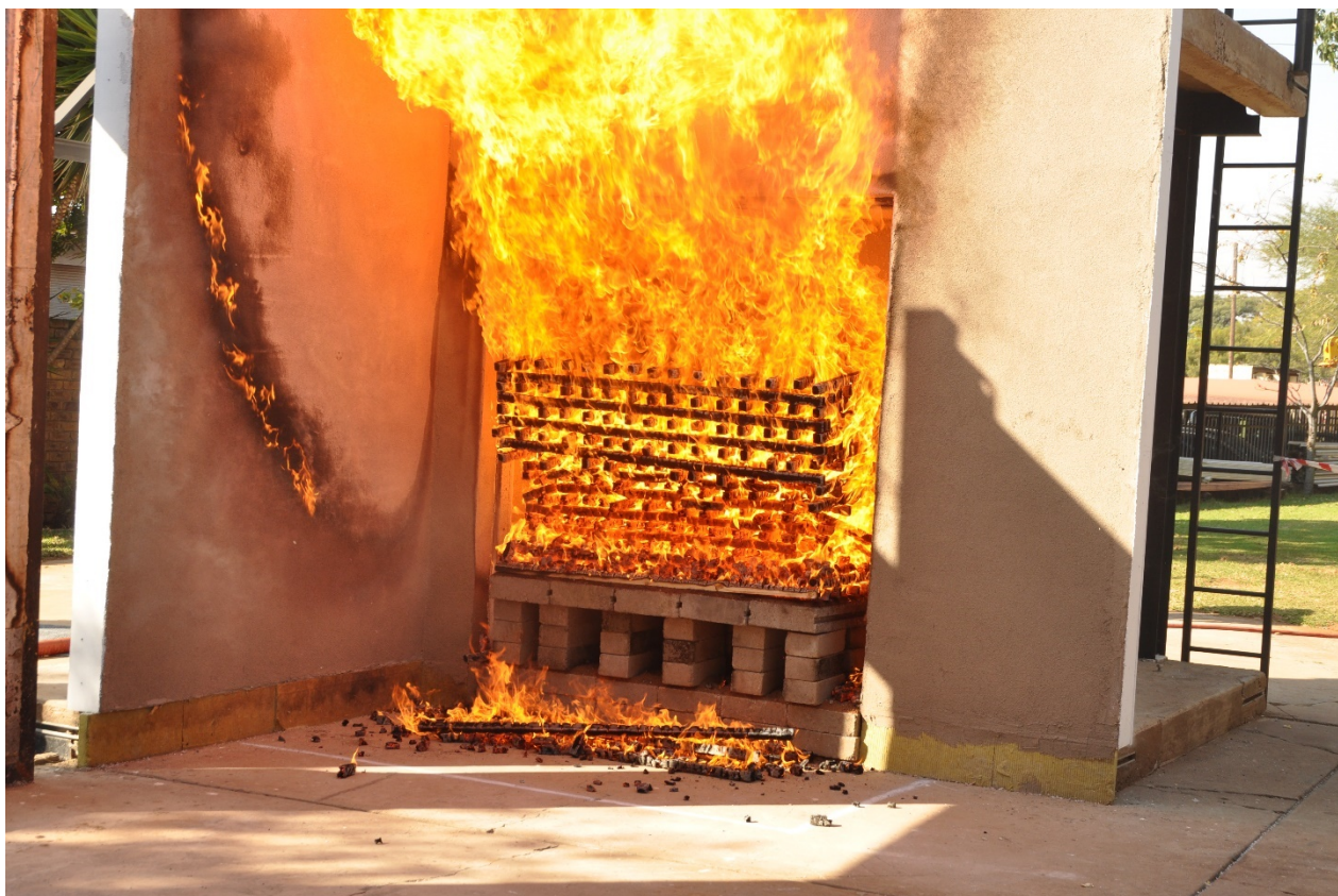
Figure 3.13: Crib starting to collapse
