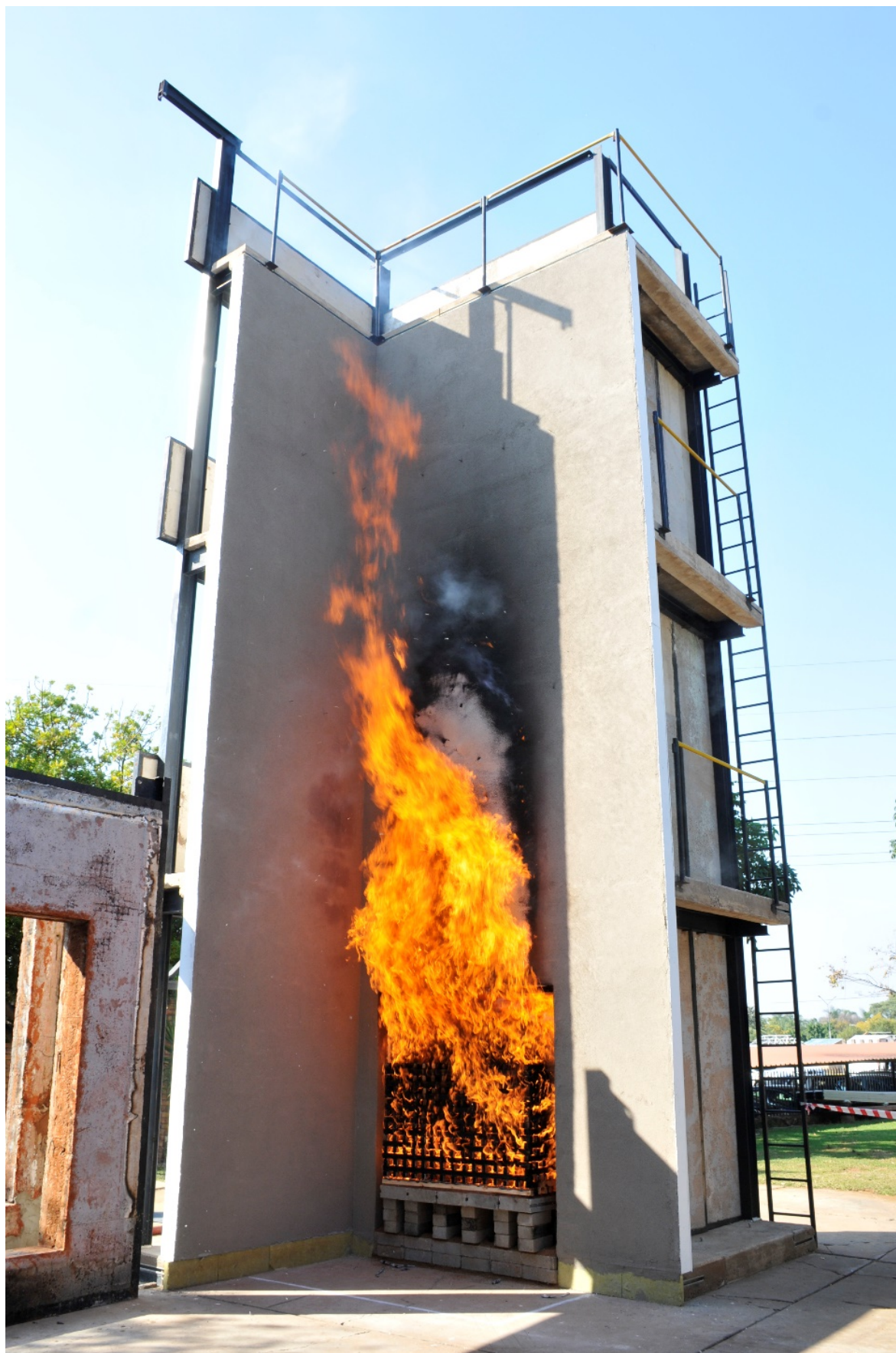
Figure 3.8: White discoloration and flames extending to Level 2
