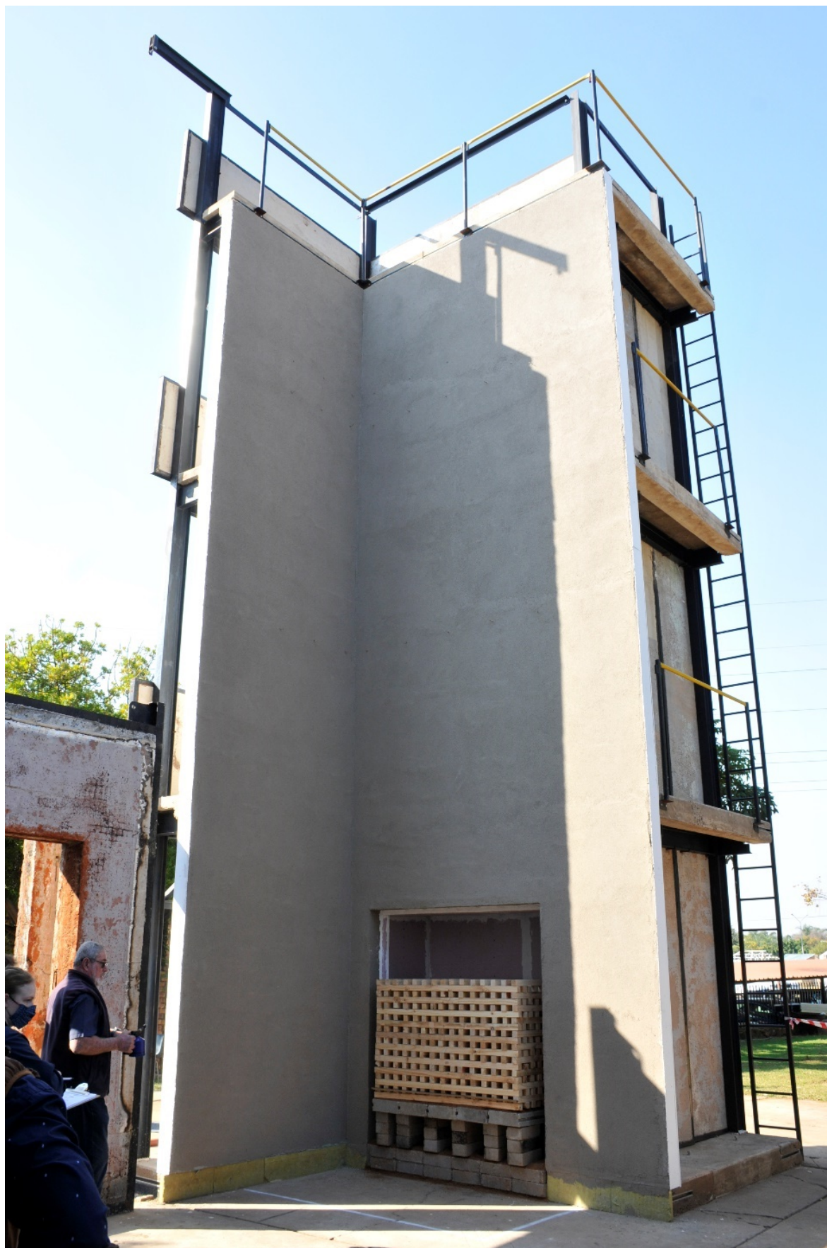
Figure 3.4: Test specimen prior to the test
