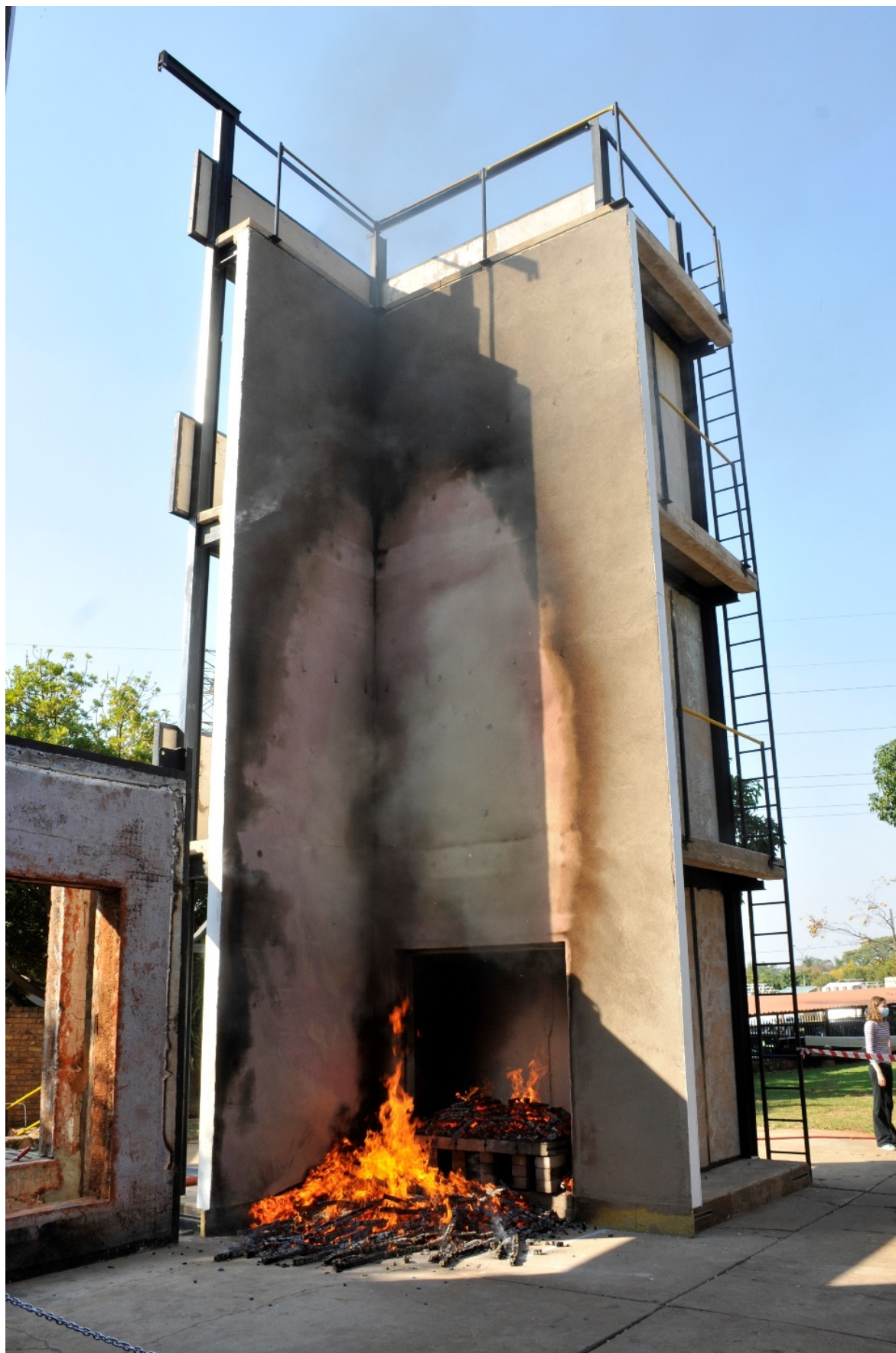
Figure 3.15: All flaming out on specimen
