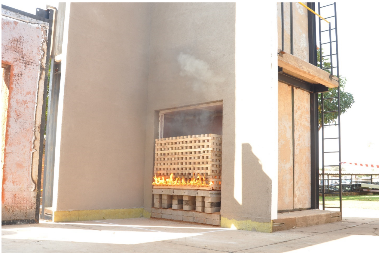
Figure 3.5: Ignition of crib (Fire Source)
