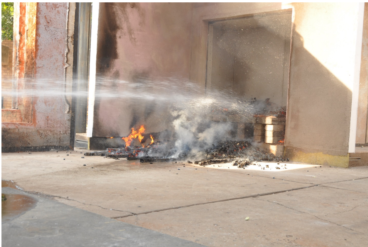
Figure 3.16: Crib extinguished (30 minutes)
