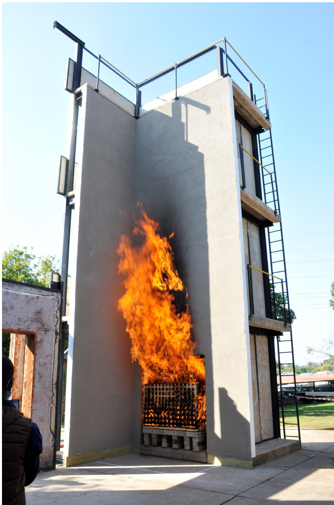
Figure 3.7: Dark discoloration and ignition on Main Wall
